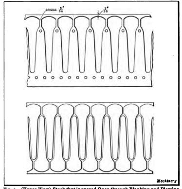
Fig. 2. (Upper View) Stock that is passed Once through Blanking and Plercing Die. (Lower View) Stock after the Second Passage through the Die
